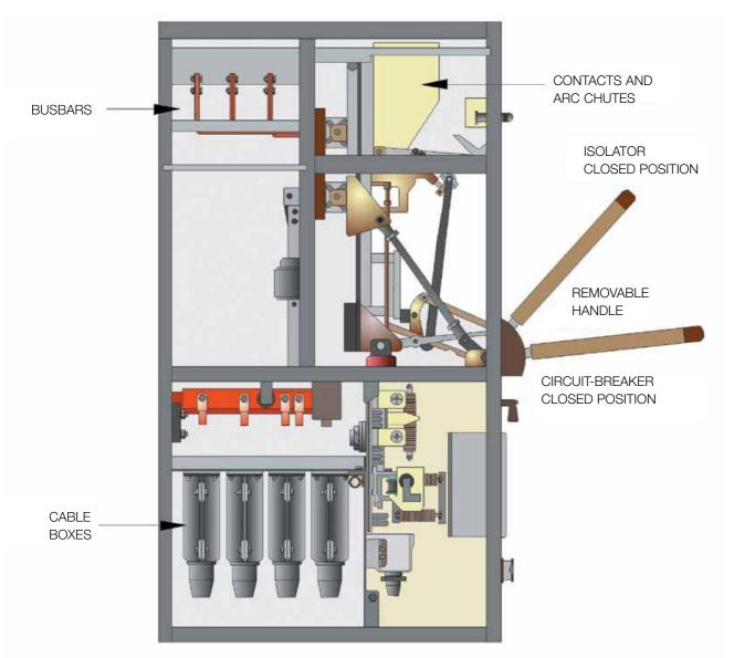
Appendix C7: Typical arrangement of a 415 V air circuit-breaker
