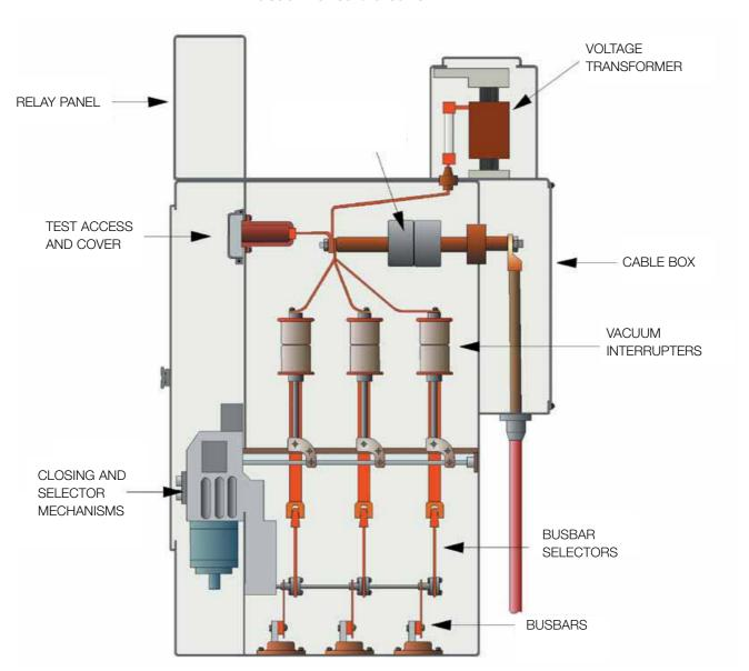
Appendix C3: Typical arrangement of a single selector fixed pattern 11 kV vacuum circuit-breaker
