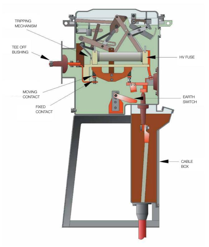
Appendix C5: Typical arrangement of an 11 kV oil fuse switch
