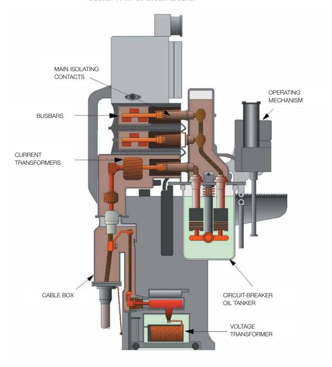
Appendix C2: Typical arrangement of a vertical isolation 11 kV oil circuit-breaker panel (single busbar with feeder earthing via circuit-breaker transfer)
